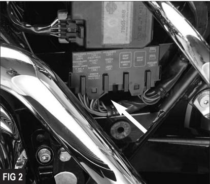
8. Remove the left block from the fuse box by releasing the catch on the front. Locate the ACCESSORY fuse located in the center, front of the block and remove it. Plug this fuse into the pigtail as shown in Figure 3 and slip the pigtail into the accessory slot.
