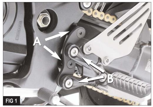
4. Secure the peg hanger to the Corbin bracket using the stock bolts at location "B", Figure 1. Tighten to 12 ft lbs and use Loctite!
