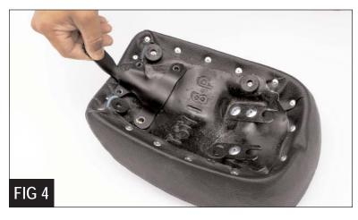
9. To install your pillion seat, slide the two rear tabs on the saddle into the two rear towers on the bike, align the front tab and secure with the stock bolts.
