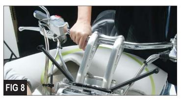
**NOTE:** These bolts are hard to reach. Using an open wrench will make it easier.
